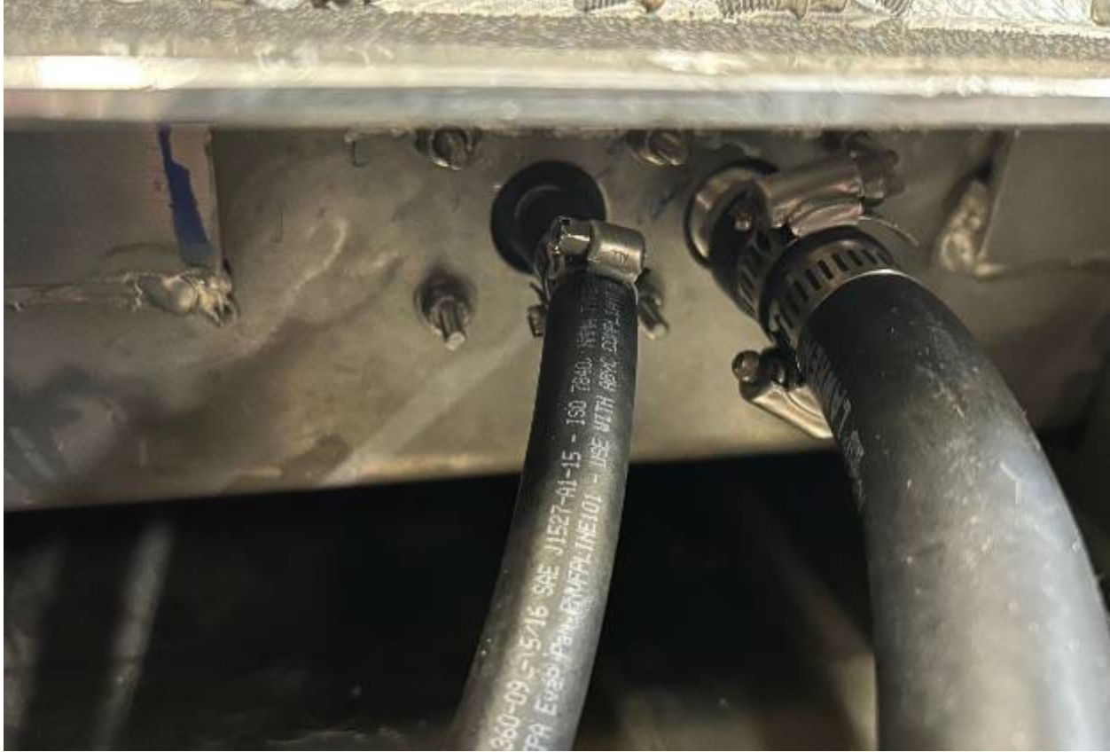
Figure 9: Ensure the vent hoses are connected to the hose barbs coming through the bulkhead and secured with hose clamps.
