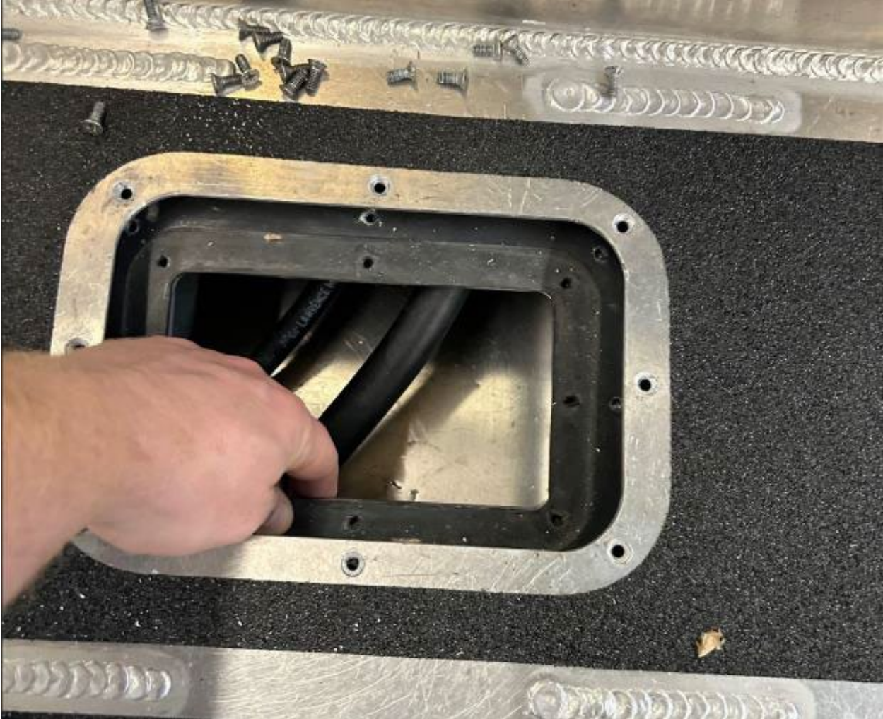
Figure 6: Remove the Phillips screws from the outside bolt circle, which hold the hatch ring to the deck. When taking the last few screws out, hold the hatch ring in one hand so it doesn't fall.
