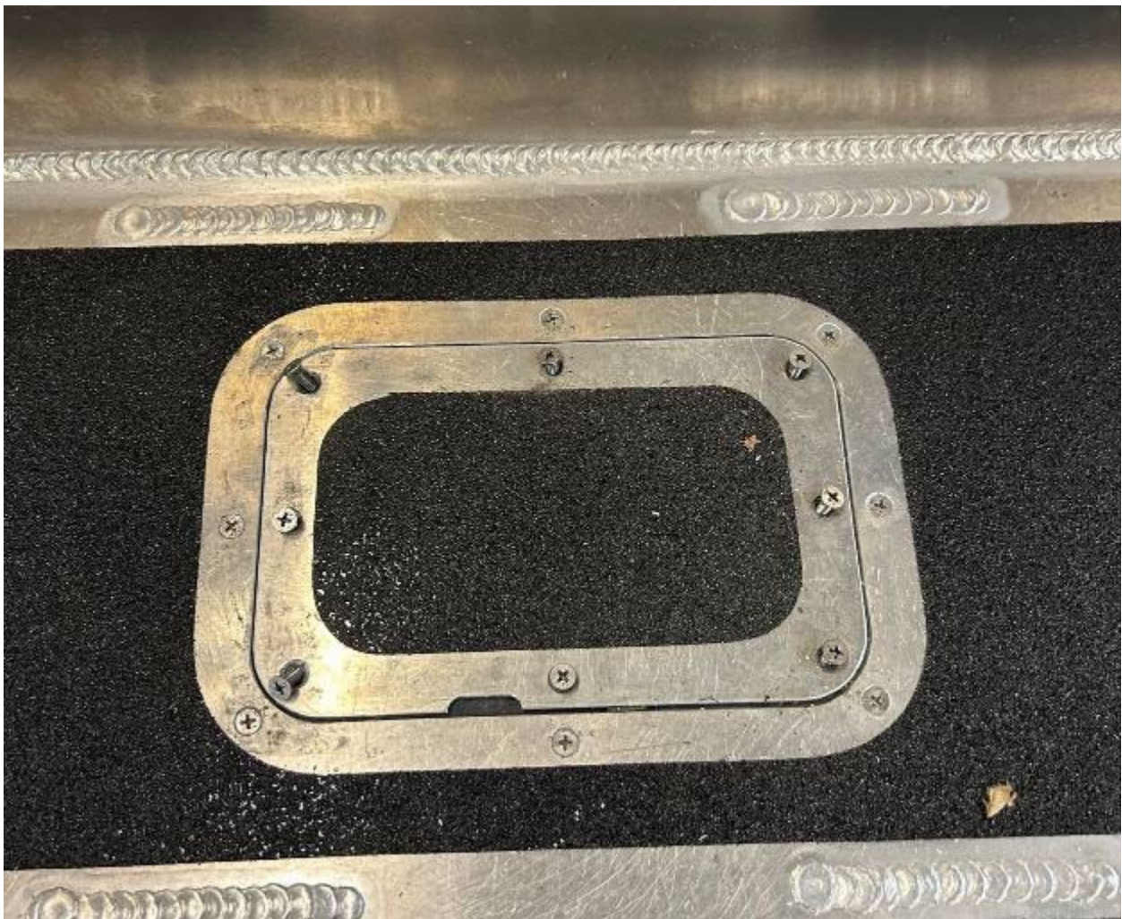
Figure 3: Remove the Phillips screws from the inside bolt circle.
