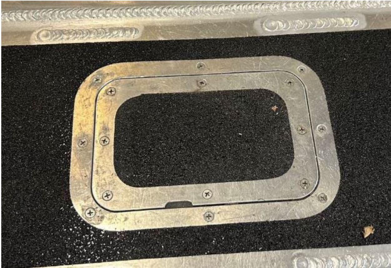
Figure 12: After installing the lid, double check that all screws are tight on both the lid and hatch ring.
