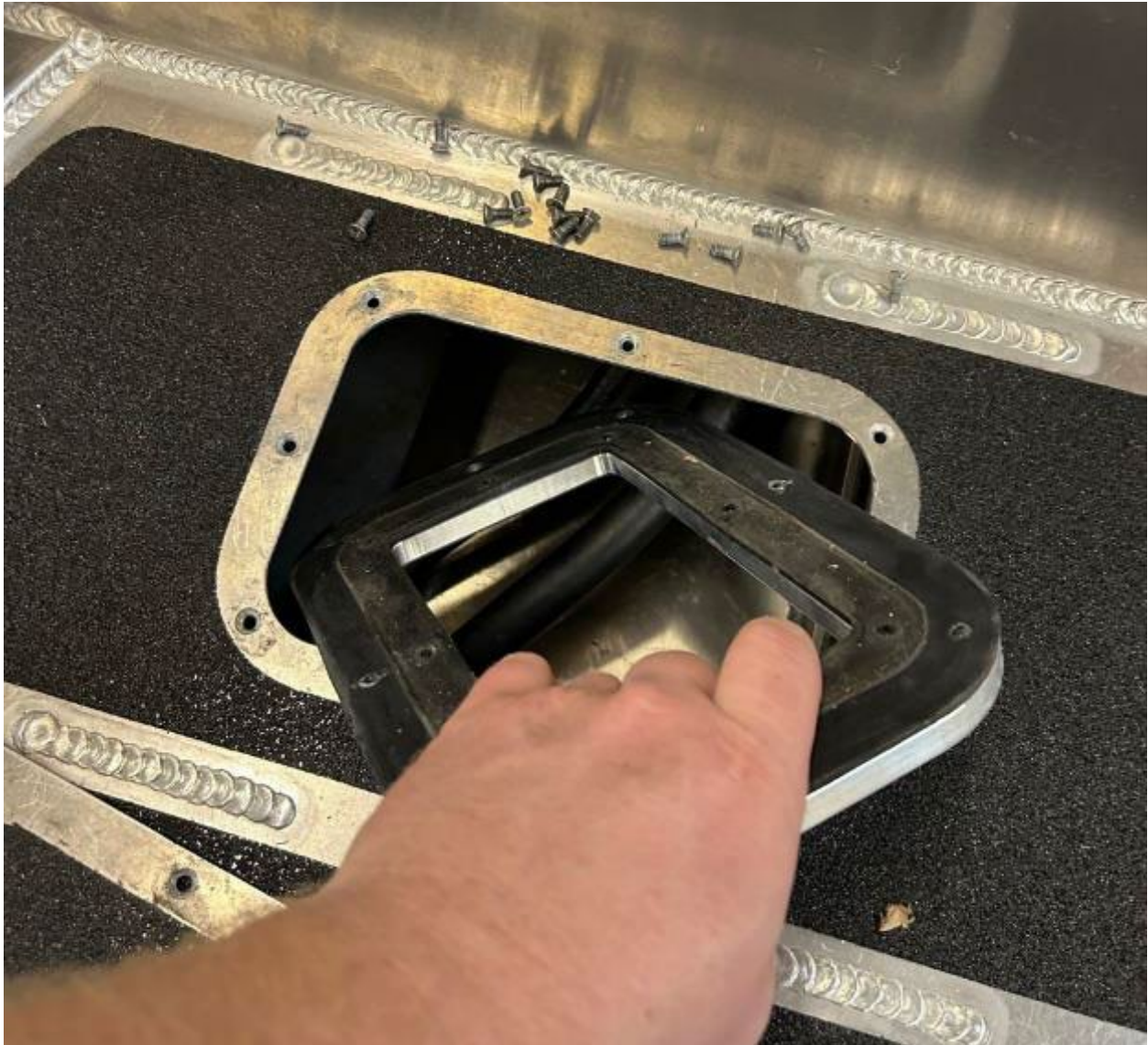
Figure 7: Once all the screws are out, the hatch ring can be lowered, rotated, and removed through the deck opening.
