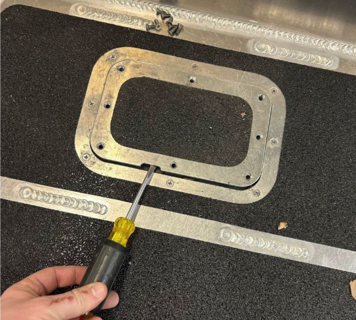
Figure 4: Insert a flat head screwdriver into the small notch to pry the lid open. Be careful not to tear the gasket below.
